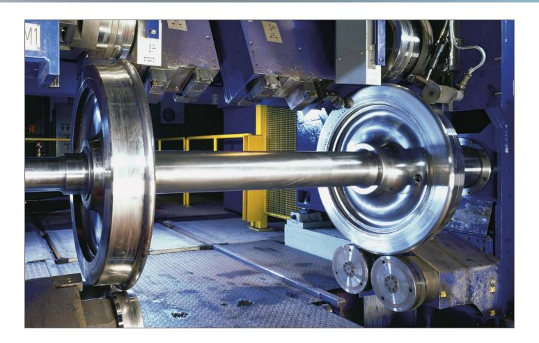
The PN 190 portal wheel lathe represents a pioneering design in the field of wheel-set maintenance. Its combination of the portal frame with the friction roller drive opens up new dimensions in the technology of wheel-set turning in terms of productivity and machining quality.
