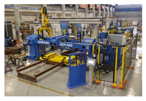
The **Simmons DDP-600 Dual End Demount Press** disassembles wheels from railway wheel sets. It has a maximum force capability of 600 tons and is capable of demounting a wheel set every 150 seconds (including loading and unloading).
