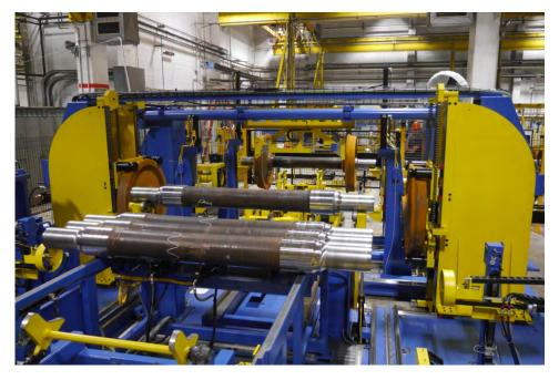
The **Simmons SMP-200 Pre-Mount and Mount Press** is a fully automatic production wheel press for mounting railcar wheels to axles. The SMP-200 takes pre-machined wheels and axles and accurately positions and mounts the wheel set in a fast, efficient, and AAR-compliant manner.
