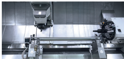
• Combination turning-milling unit and tool carrier
