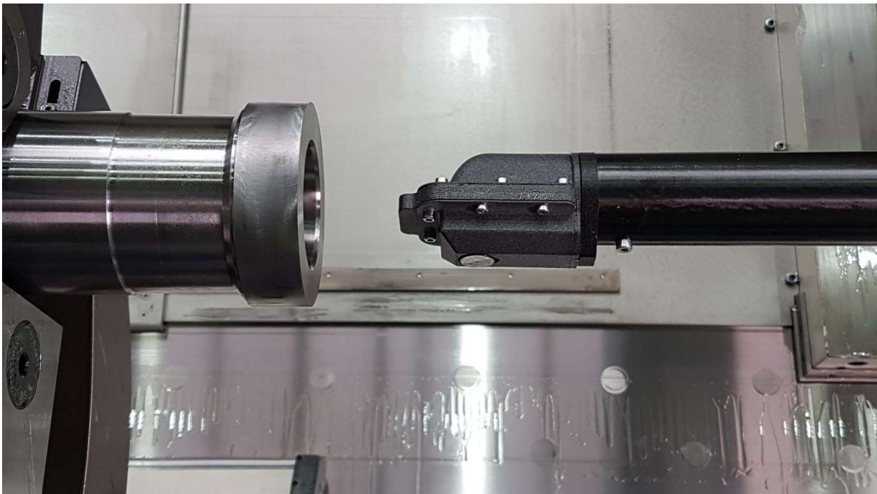
Image 4 - Eddy Current Sensor for Determining the Optimal Workpiece Center Axis
