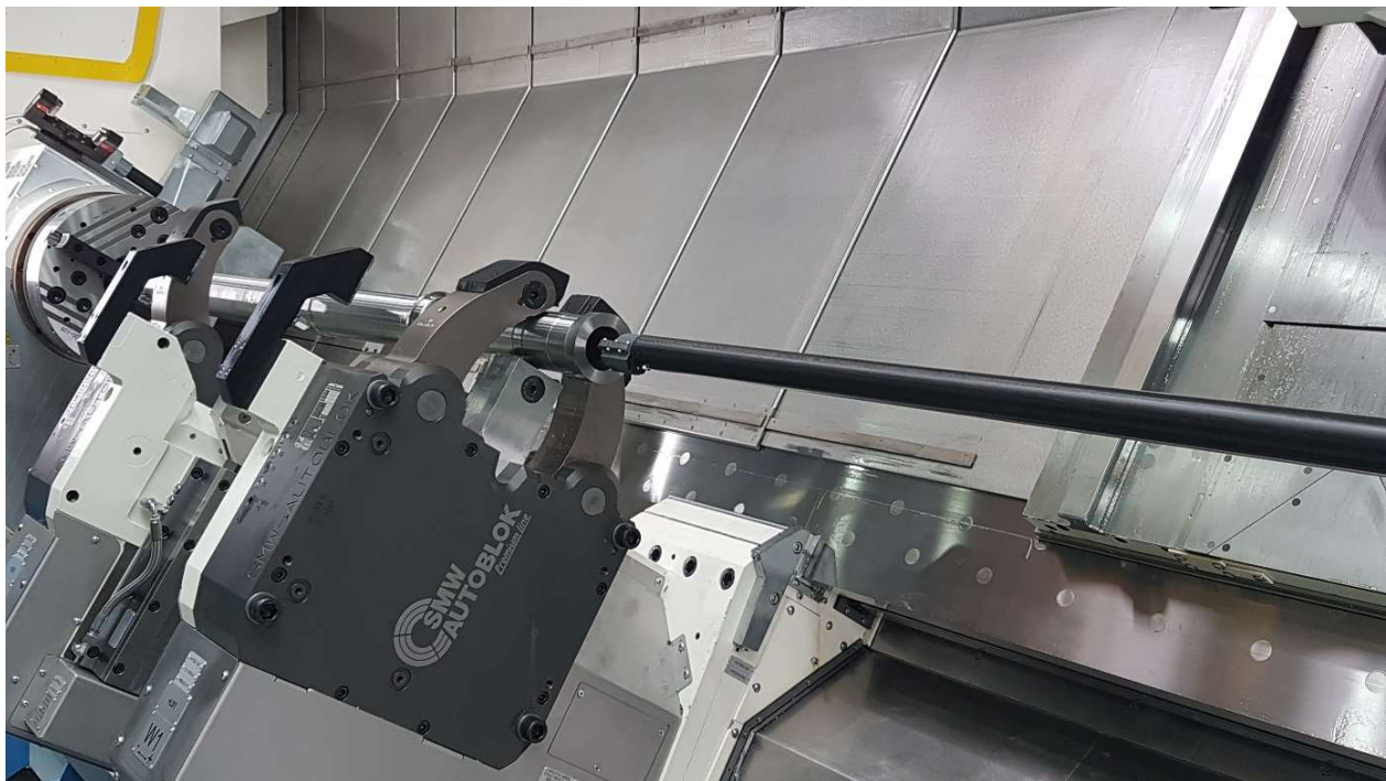
Image 5 - Carbon Measuring Lance in the "CENTER AXIS ALIGNMENT" Process
