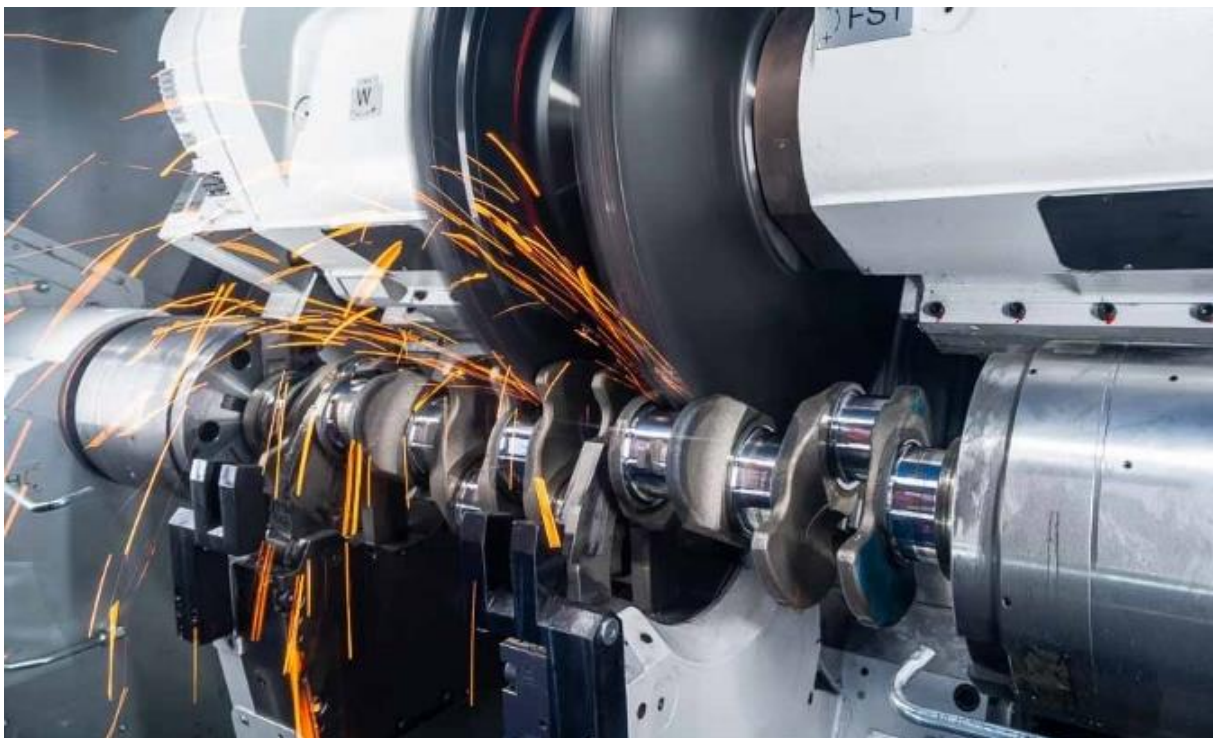
Image 1 - Hard milling of a 6-cylinder crankshaft for trucks
