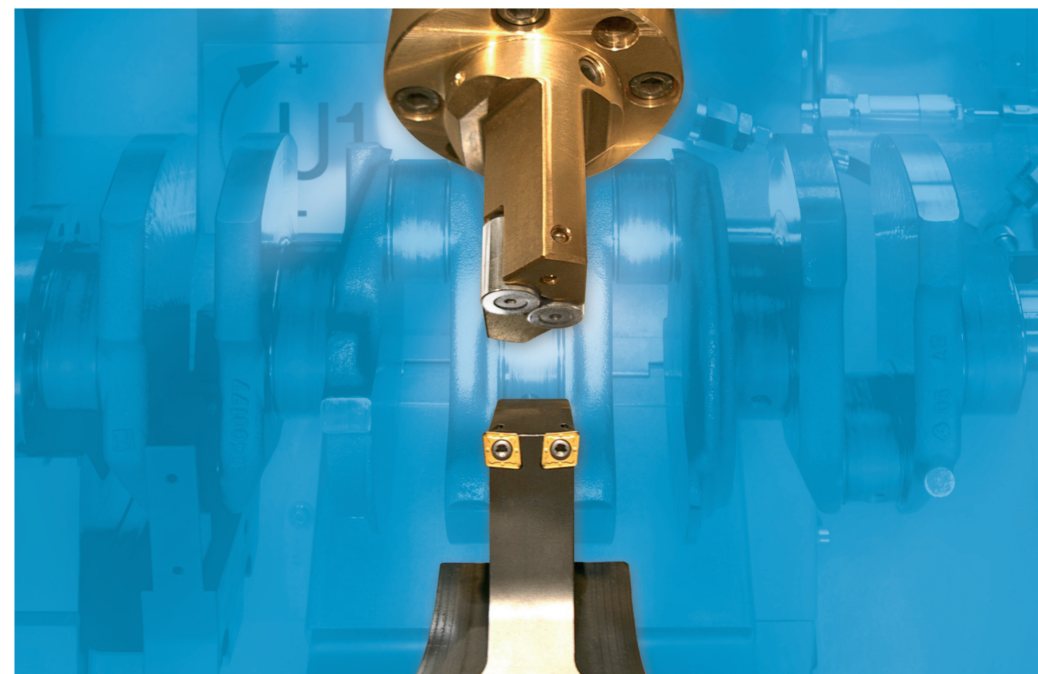
For serial processing of crankshaft thrust faces and flange faces
