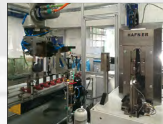
Machine-integrated RASOMA-articulating gantry loader and measuring station
