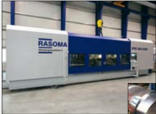
EBZ 400-4500 for end- machining large crankshaft of up to 4,500 mm in length
