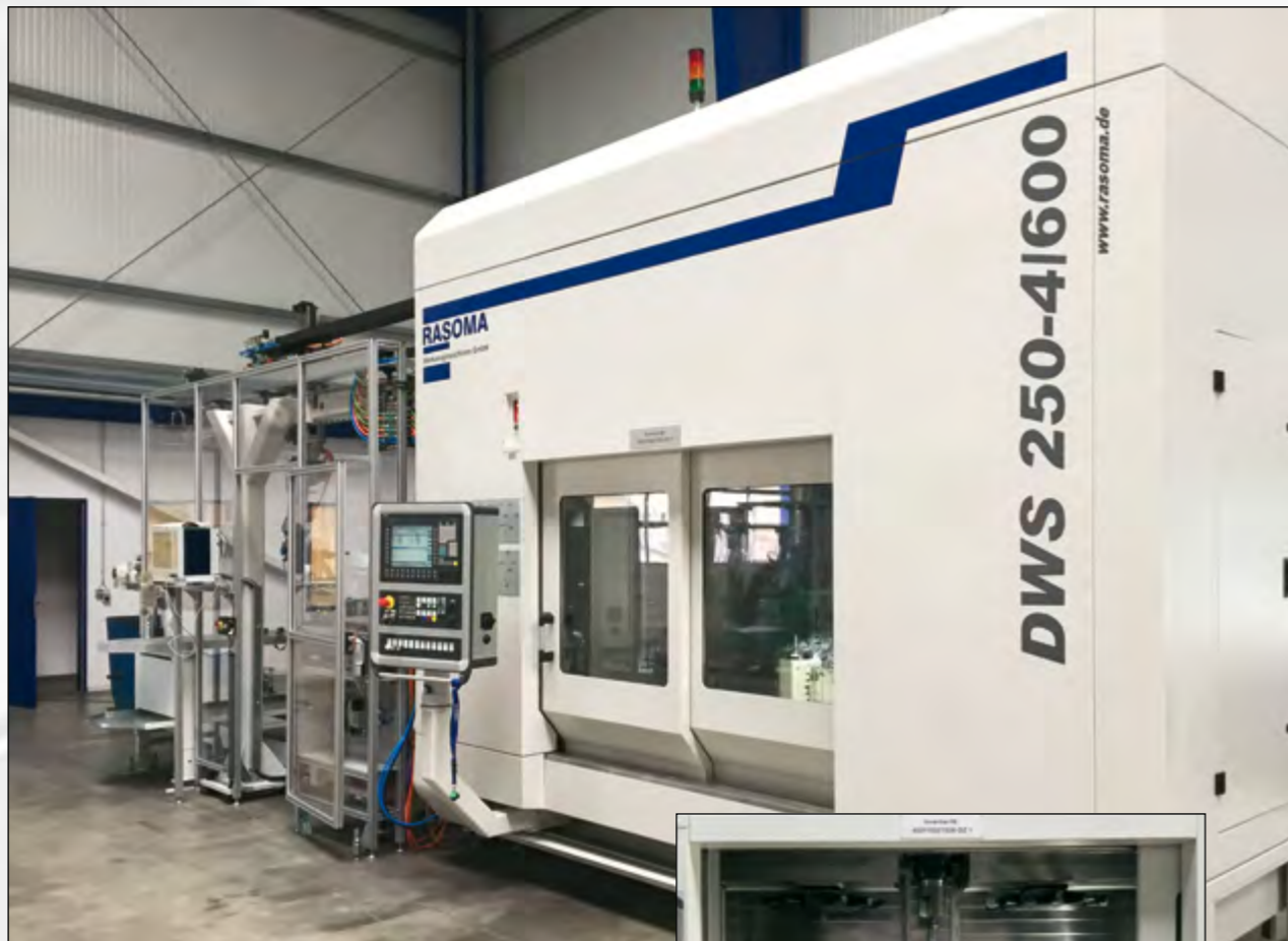
RASOMA Vertical-shaft turning center DWS 250-4 with automated supply and removal of work piece
