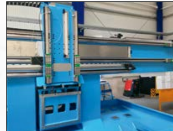
The base frame of the machine with longitudinal slide on three linear guides, cross slide for suspended, pivoting tool spindle. Below the Y-slide with bolting surface for the clamping device
