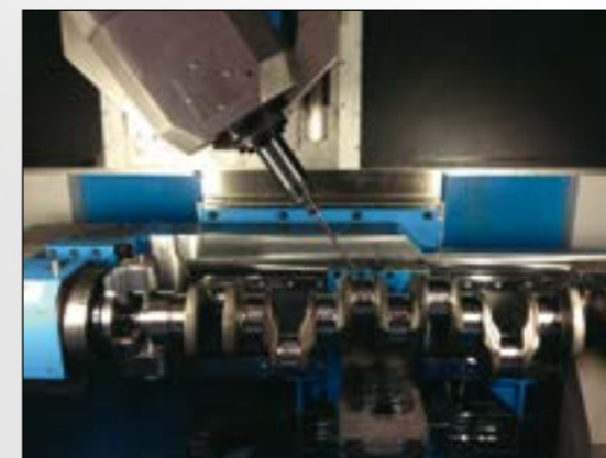
Infinitely tilting tool spindle and clamping device with turning module and C-axis, movable tailstock and programmable steady rest in support of processing prolonged crankshafts
