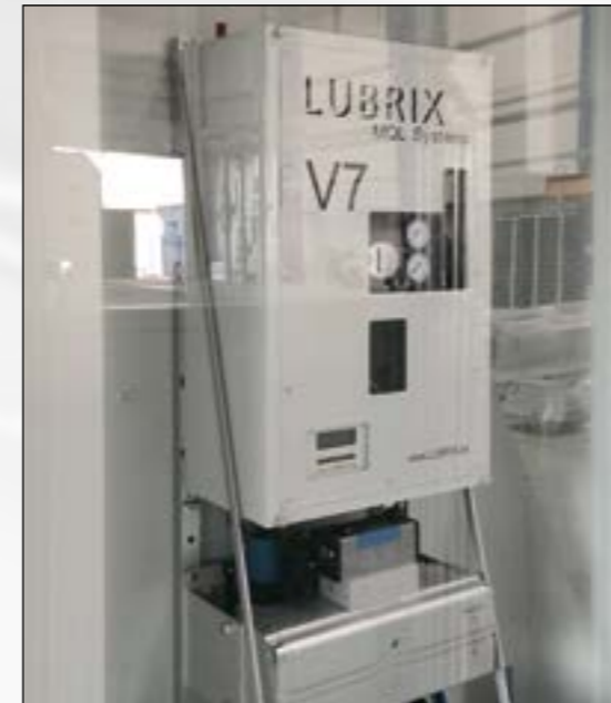
Minimal quantity lubrication causes optimal cutting values during deep hole drilling and is decisive for a high productivity. In addition, it fulfills cost saving in comparison to the classical application of high pressure cooling lubricant systems
