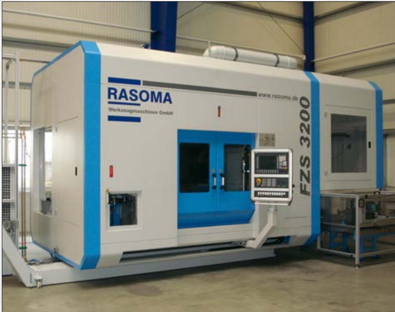
Our newly developed modular constructed CNC manufacturing center FZS 3200 is especially qualified for processing oil drilling and weight reducing holes of crankshafts or similar undulated parts of up to 1,150 mm in length
